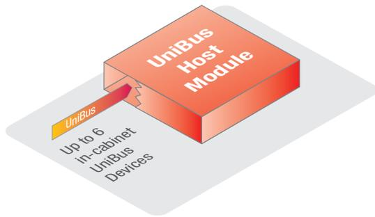
UniBus Devices are designed for installation within the same enclosure as the UniBus host module. A UniBus host can interface a maximum of six UniBus devices in any combination, provided they are all within the intended functionality of the host module
