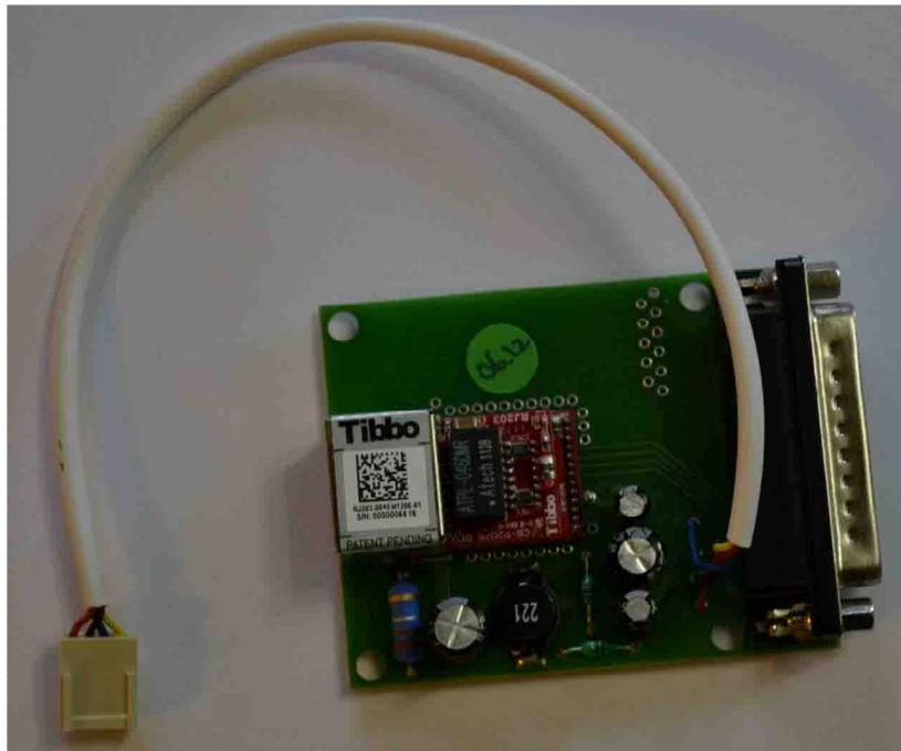
Please connect 4-PIN connector to Paradox panel serial port and RJ45 connector into LAN. The IP module receives its power from Paradox panel.
