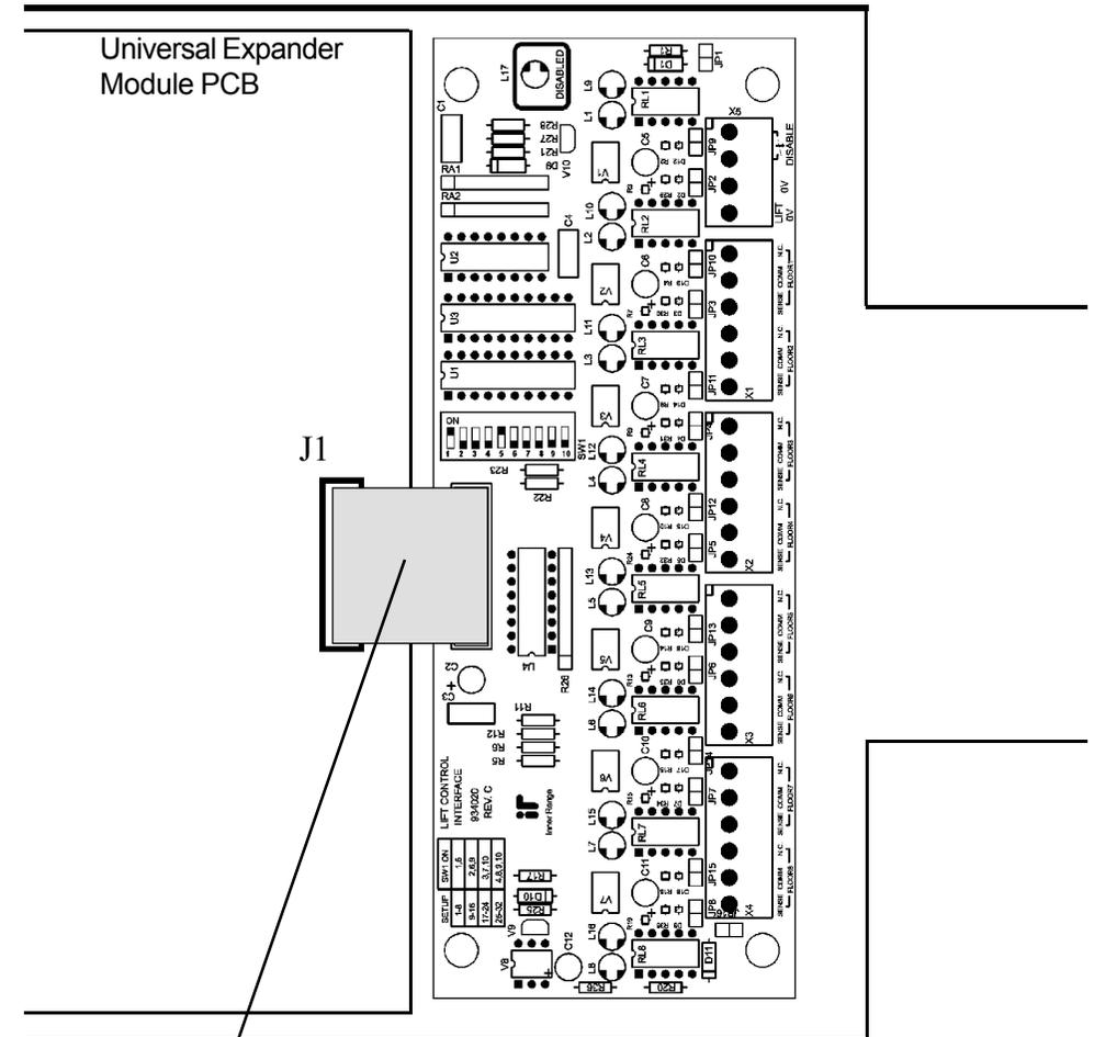
Lift Interface board connected to Universal Expander with ribbon cable supplied.
