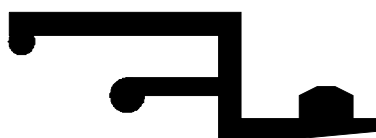
Flush mount option. Top of Plunger removed.
