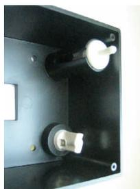
Location of the tamper switches in the plastic enclosure
