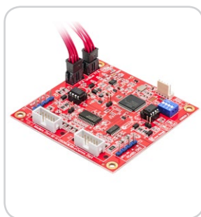
Integriti UniBus 2 Port RS-232/RS-485 UART PCB & Accessories (Includes 270mm UniBus patch cable) Part 996520PCB&K
