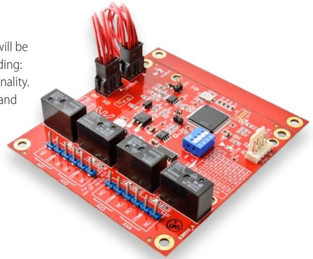
*“UniBus is an innovative in-cabinet bus which allows the connection of Expansion modules, Communications modules and even Door & Reader modules on a common Plug & Play bus. UniBus is built on the highly reliable CANBus technology and replaces the need for ribbon cables and specialised connectors”*
