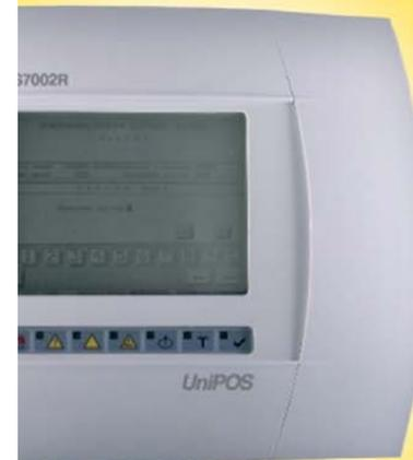
The IFS7002R Repeater panel provides additional indication and control for fire alarm systems based on addressable Fire Control Panels IFS7002. The function of the repeater is to exchange information and control commands with one or more addressable Fire Control Panels IFS7002 and other repeaters connected in a local area network.
