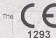
The marking may only be used if conformity with all relevant and effective Directives of EP and Council is attested.
